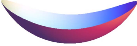
FIG. 4. (Color online) The n=2 mode. The dominant instability encountered in a thermodynamic stability analysis. The elongation of the shell allows relaxation of the perimeter stress.
